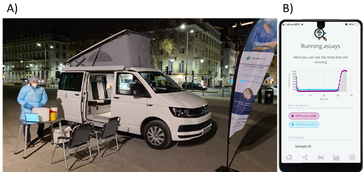
Figure 4. COVID-19 testing at point of care (downtown of Lisbon, Portugal) using the pocket-sized isothermal lab-on-phone COVID-19 assay (A), which can display results in real-time through a mobile app for up to four devices simultaneously (B).
