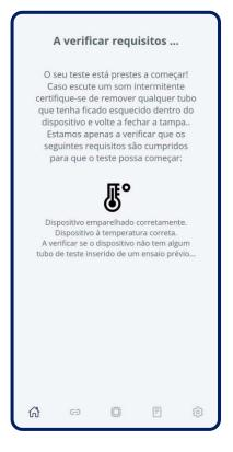
After selecting the "Start test" button, the system will check if the requirements necessary to start the test are met. Make sure that the device does not have any test tubes from the previous test. If so, you will hear a beep. Please take it off to continue.
